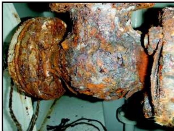
Corroded ship side boiler blow down valve
