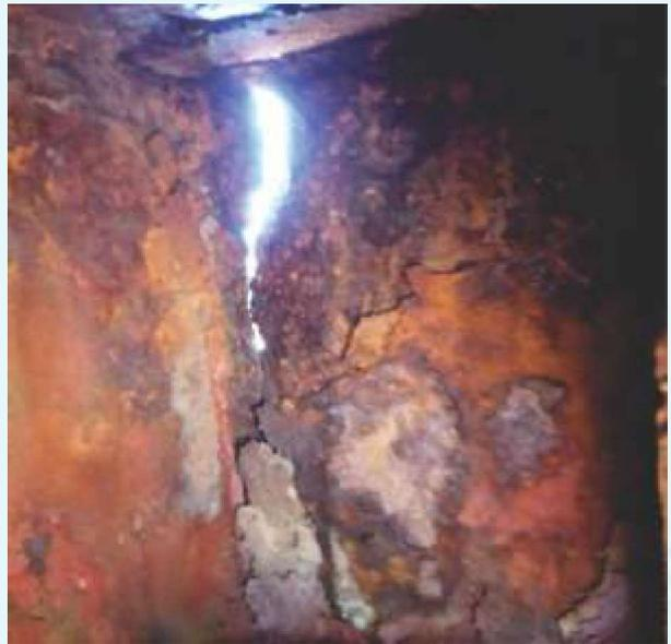
Hatch Coaming Crack
