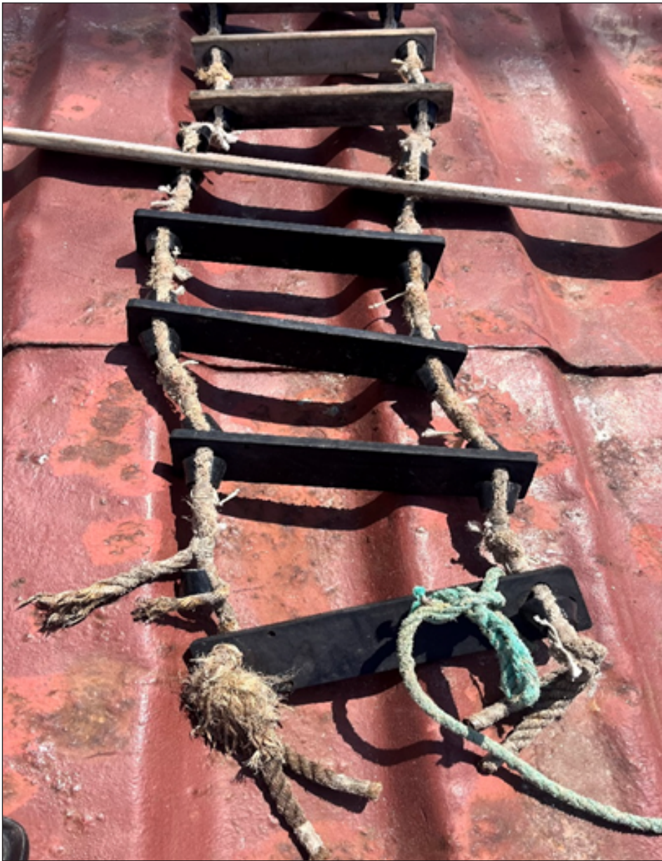
Pilot ladder was unsafe. (rope and steps) [unsafe]
