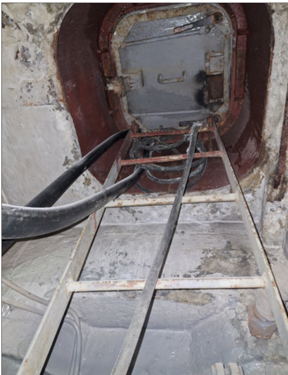
Emergency Exit Way in Pump Room Obstructed by Flexible Pipe. [unsafe]
