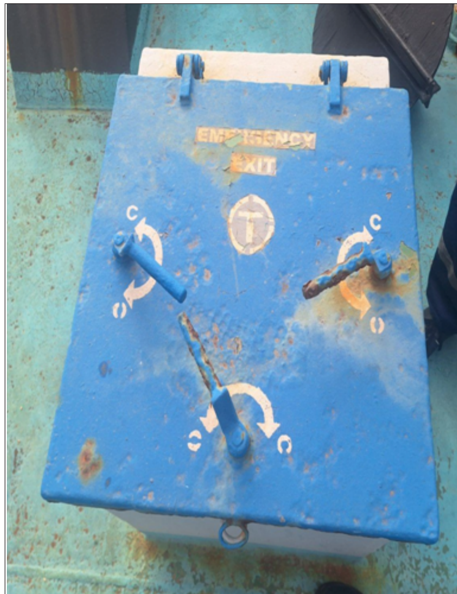
Door Handles of Forecastle Emergency Exit Way Seized. [not properly maintained]
