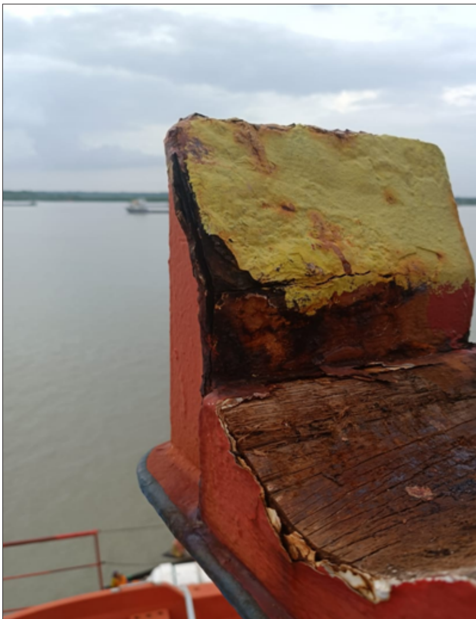
Resting Pedestal for the Provision crane found Rusted & Corroded.
