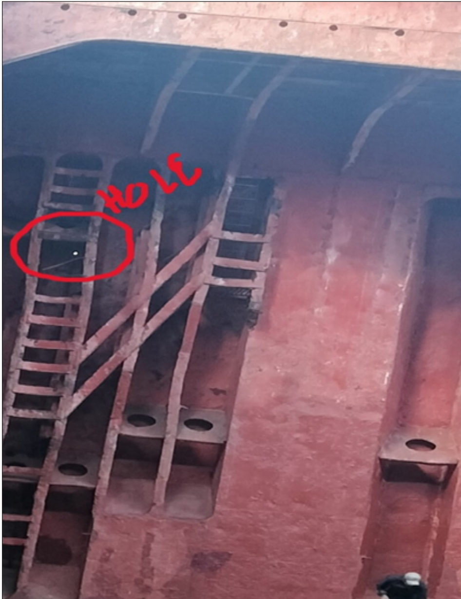
Cargo holds corroded with cracks and holes [damaged]
