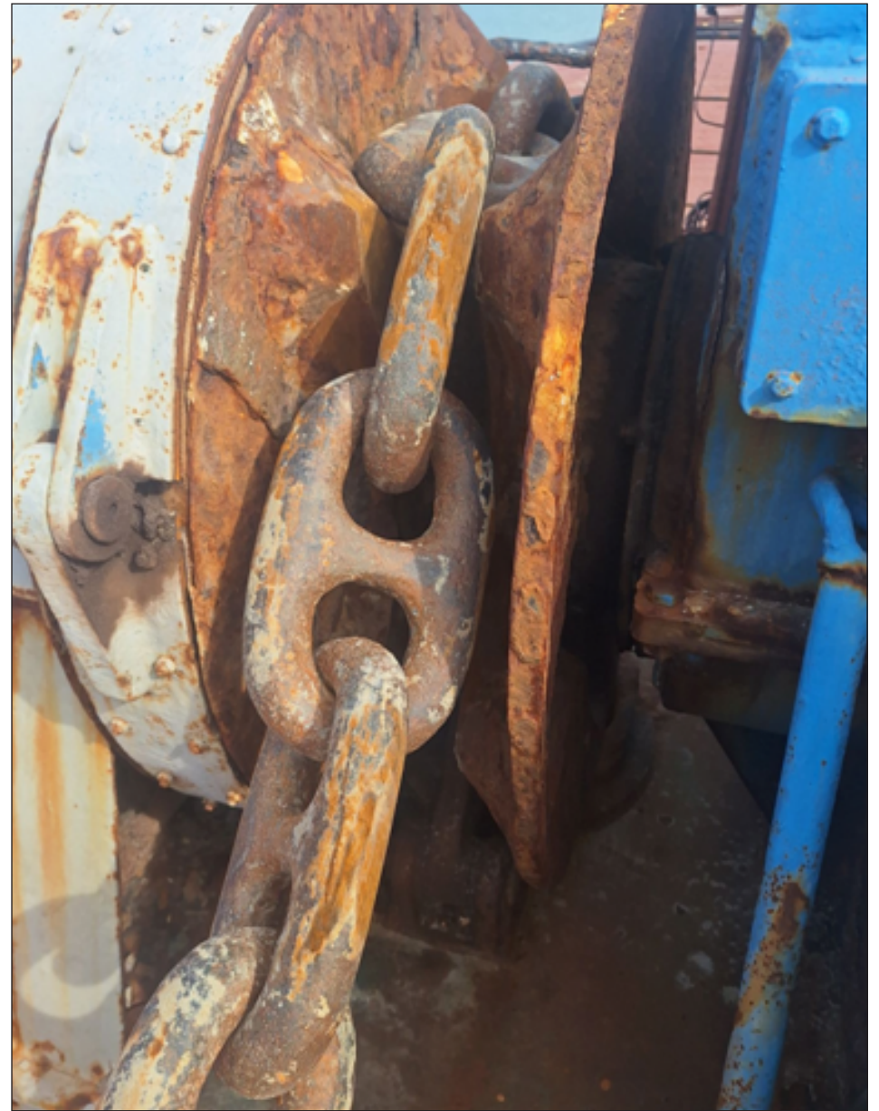
Both Sides Anchor Gipsy Wheels and Mooring Capstans Corroded Heavily. [Not properly maintained]
