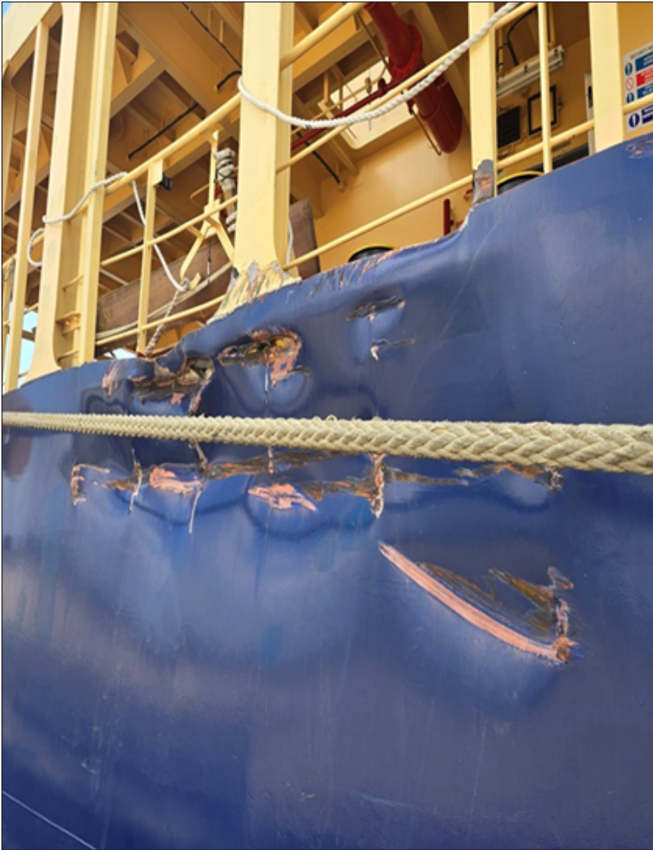
Pierced a hole in the hull between Frame No 5 to 10.
