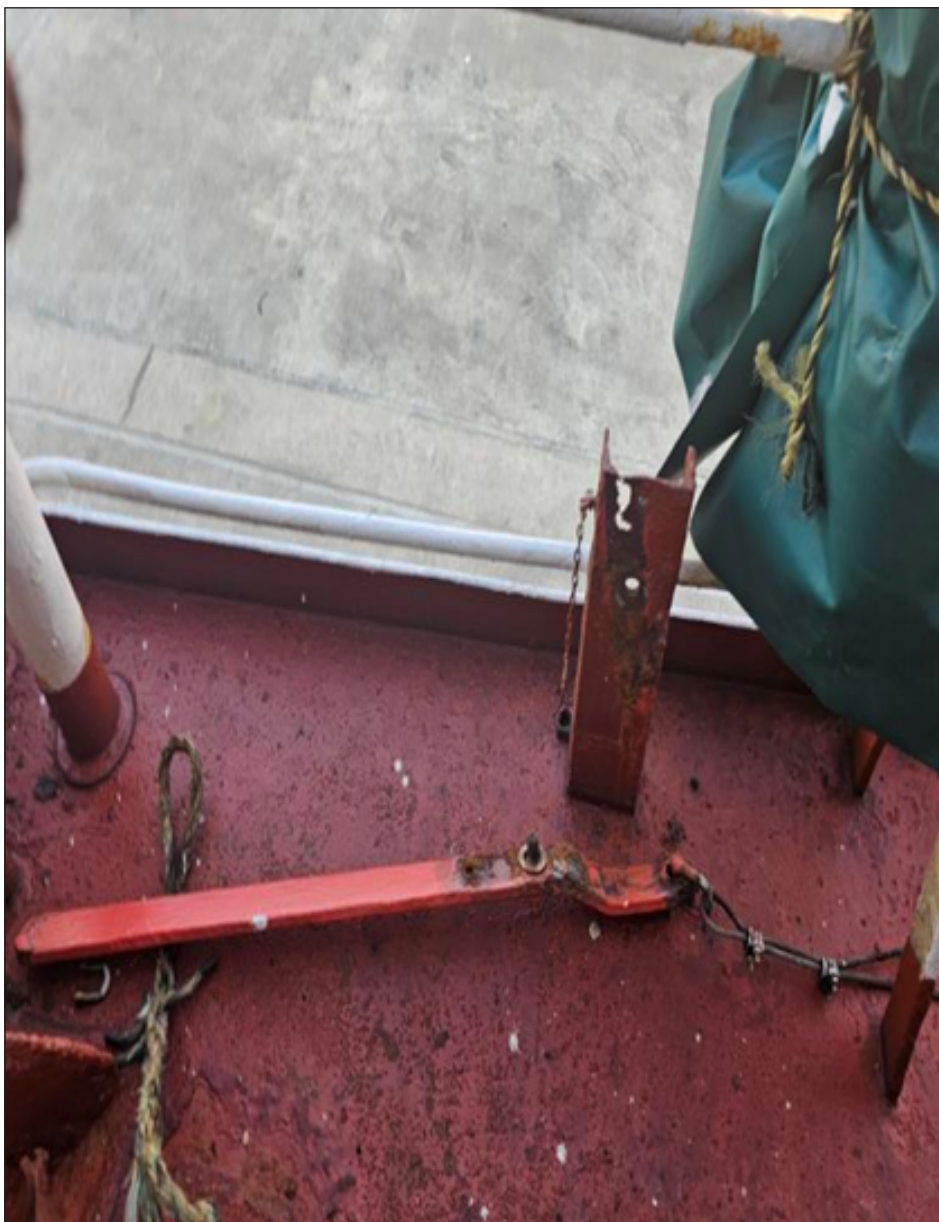
Remote launching handle from port side life boat wasted and detached [Damaged]
