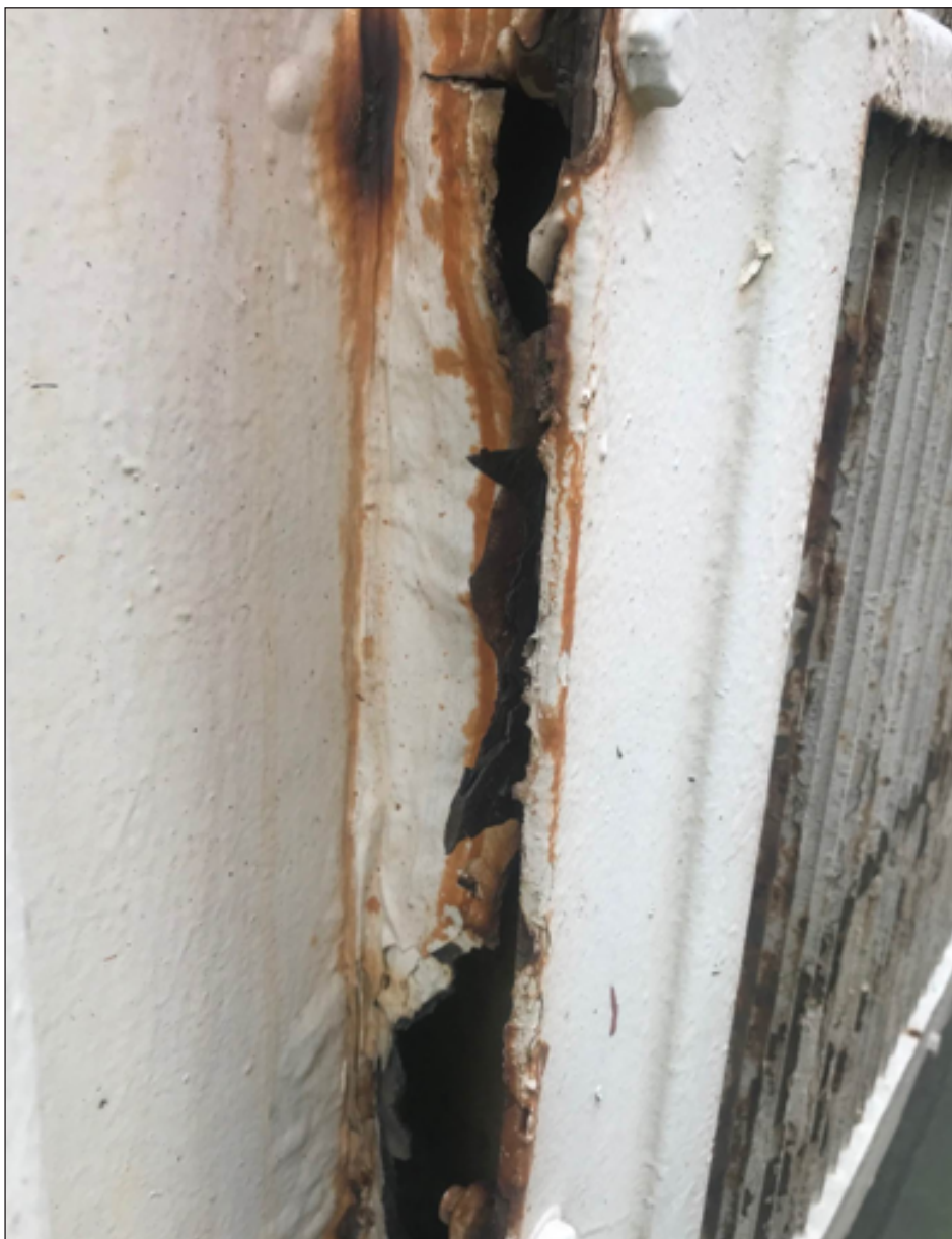
Engine room aft blower's inlet fin frame found completely corroded and wasted. [corroded]
