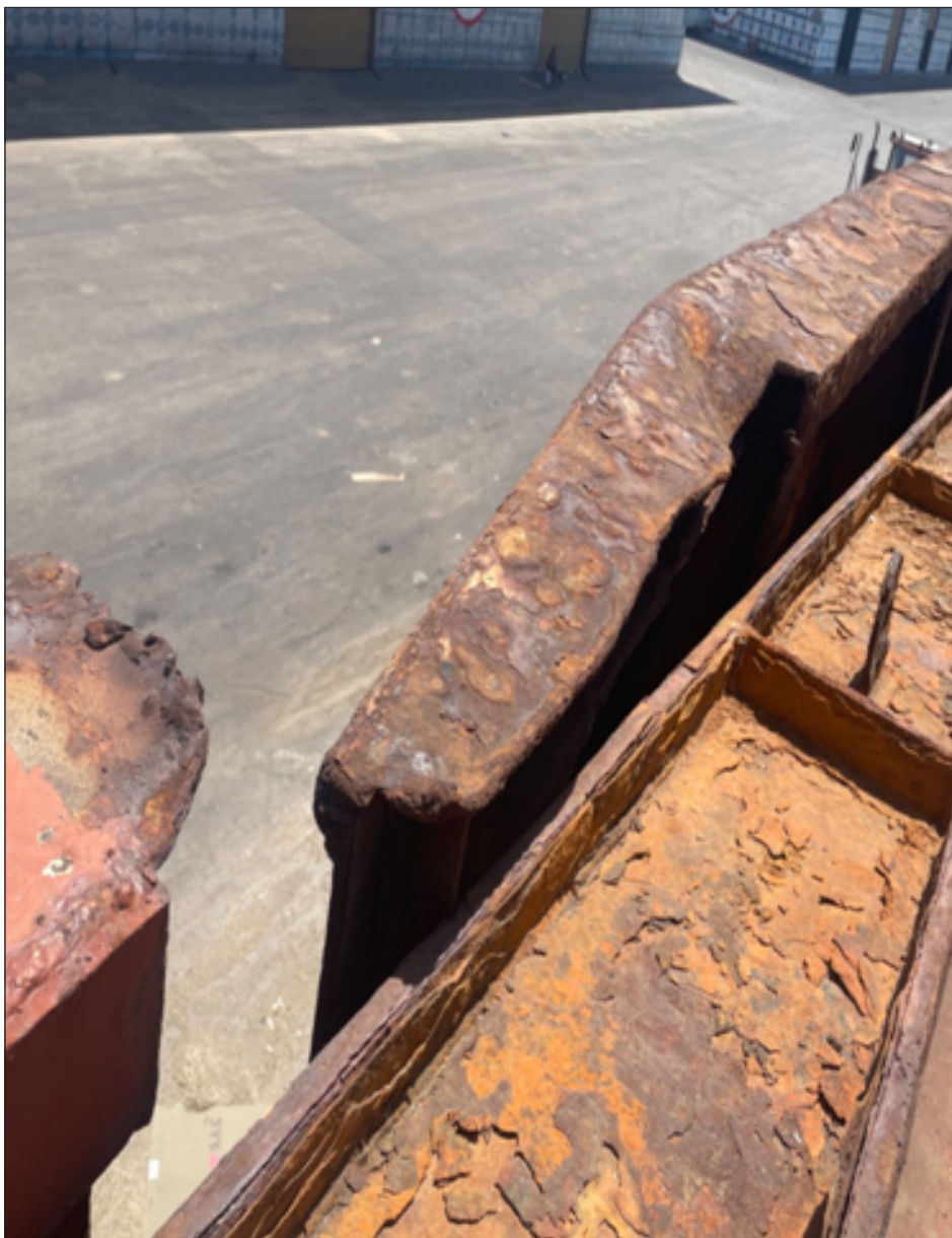
Bulwark & guard rails corroded & broken [damaged]
