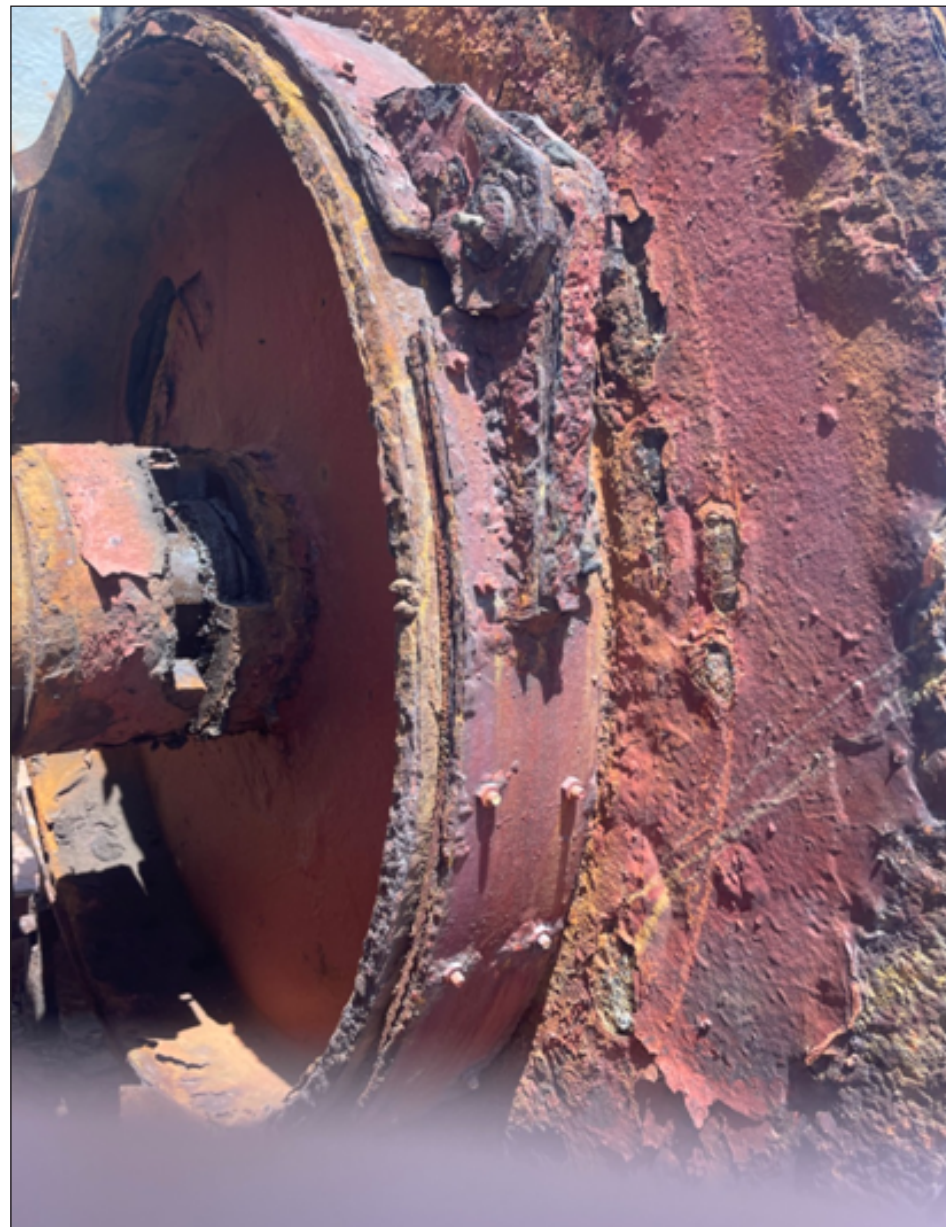
All mooring wings bed plate & drums heavy corroded [corroded]
