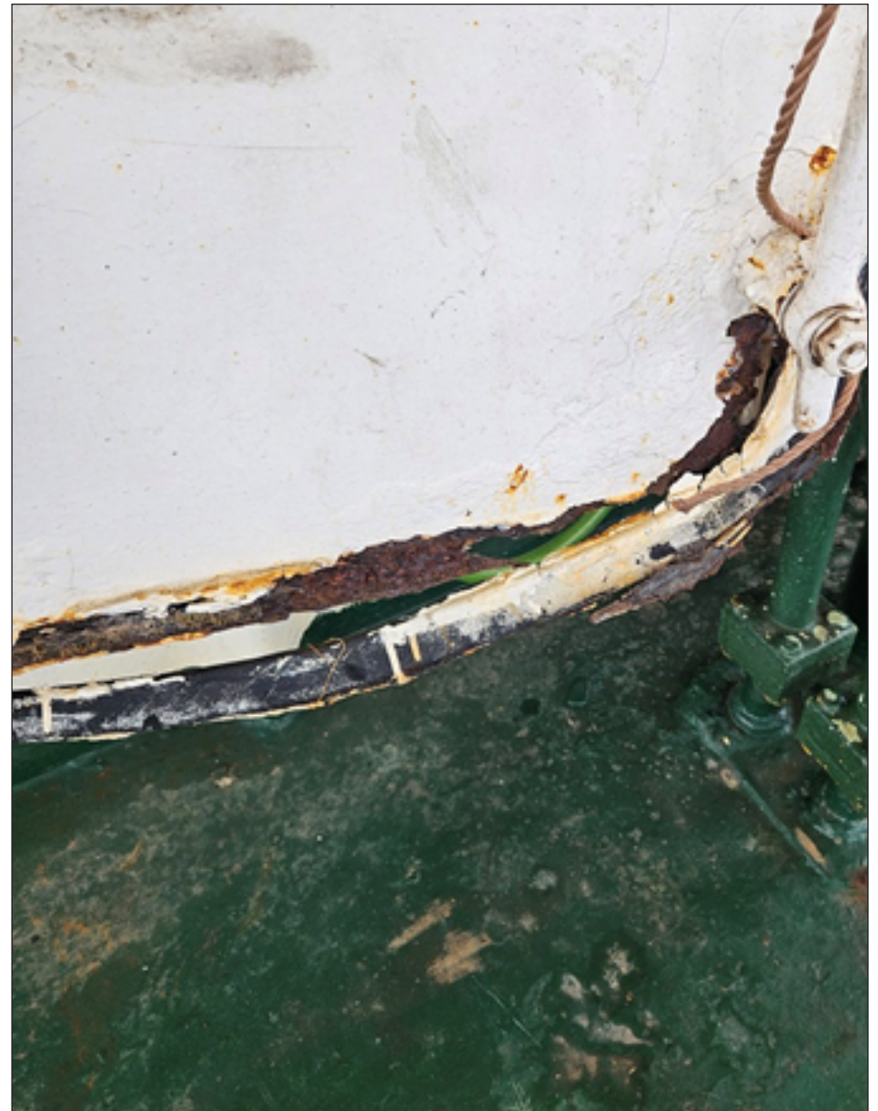
lower part of Engine room entry weathertight door from aft side (outside of the accommodation) are wasted and holed. [cracked]
