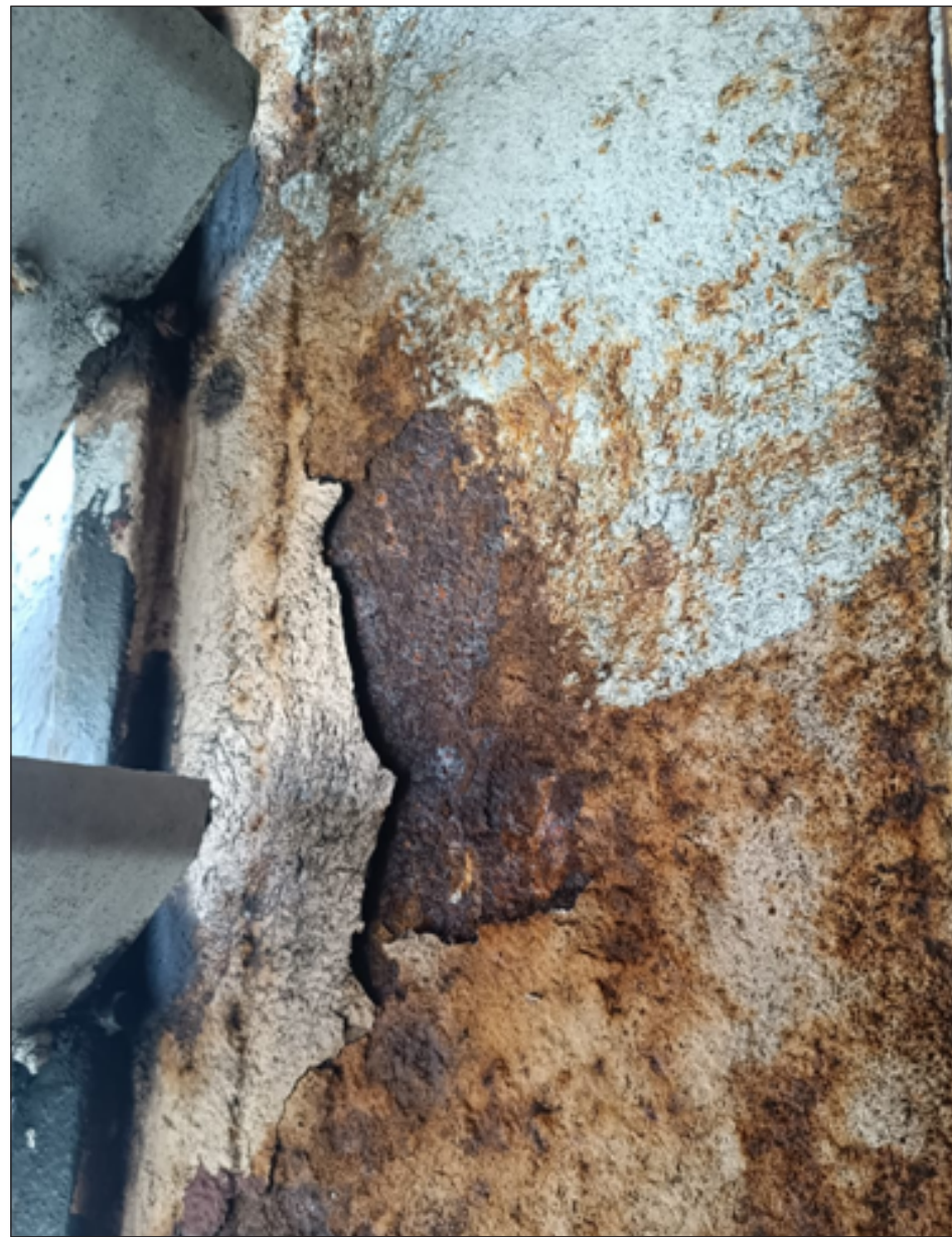
Base plate for Life Boat found Rusted, Corroded, thinned and Holed in some Places
