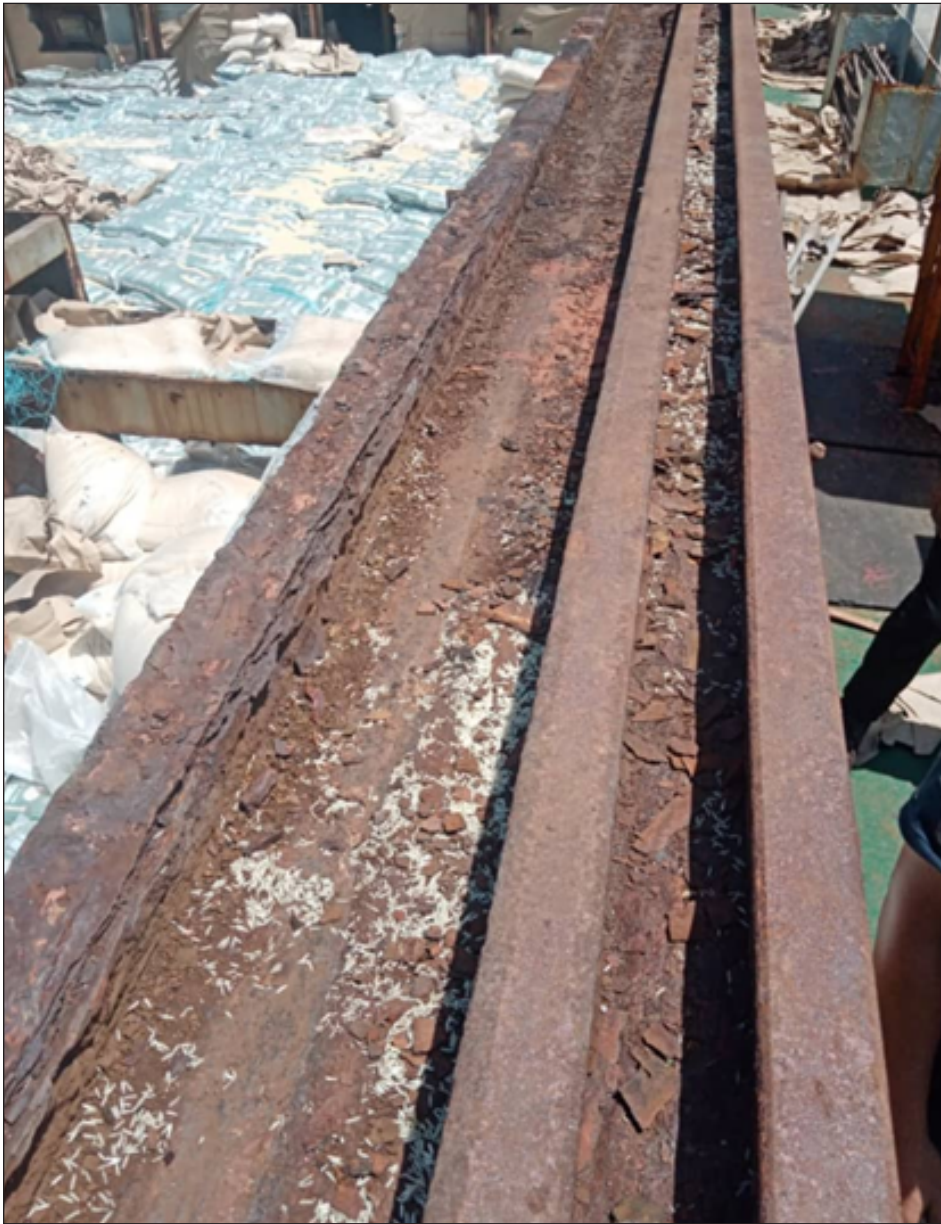
the top end of hatch coaming No. 2-3 is very rusty and corroded [Other]
