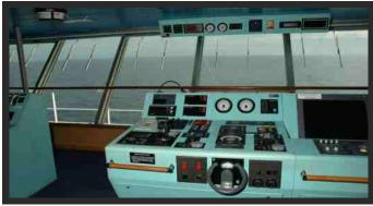
Communication between the bridge and the steering gear room, and rudder indicator tests are frequently checked by PSC
